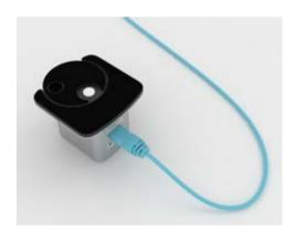
**Illuminance:** Place the connected sensor with the diffuser in the direction you want to measure, and with illuminance selected on the sensor wheel.
