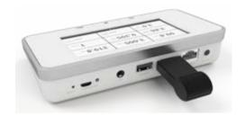
Connect the Bluetooth adapter to a SENSOR port on the base unit. A gray Bluetooth status symbol appears in the upper right corner of the screen.
