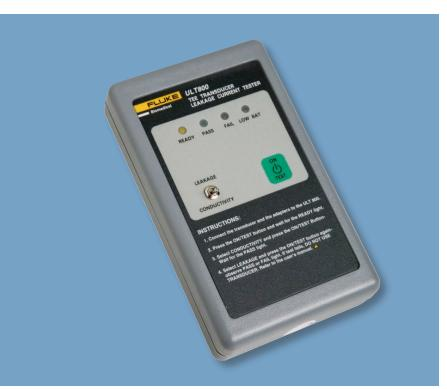
ULT800 tests the electrical safety of ultrasound transducers independent of their ultrasound machines. A variety of adapters allow for testing of many different makes and models, including transesophageal echocardiography (TEE) transducers.
