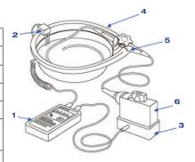
Using the ULT800 with disinfecting/testing tray and the 600/220 Dual Conductivity Probe to test a TEE transducer.
